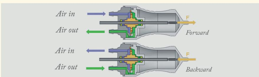
Figure 3. With spring-driven pneumatic probes, the higher the cut rate, the greater the probability of the port being closed by the cutter, making maintaining a constant flow rate a real challenge. With Oertli's dual pneumatic probe, one pneumatic pulse pushes the guillotine, while the second pulse pulls. This means that 50 percent of the duty cycle can be maintained at cut rates of 5,000–10,000 cpm.
