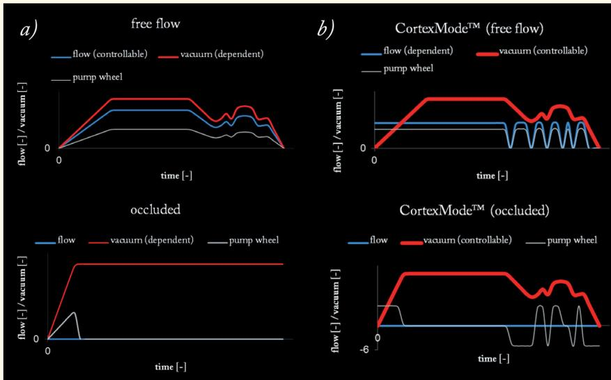
Figure 1. a) Flow and vacuum performance over time using a standard peristaltic pump mode for ophthalmic surgery. b) Flow and vacuum performance over time using Oertli's CortexMode™.
