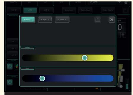
The OS4's LED light control screen, allowing the user to alter the color and intensity of the lights.
