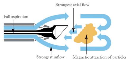
Once there, the fragments can easily be aspirated (image). The phaco energy is directly transferred into the nucleus.
