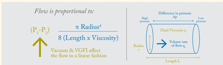
Figure 2. Poiseuille's Law of total volume that flows through the tube: vacuum affects the flow in a linear fashion.
