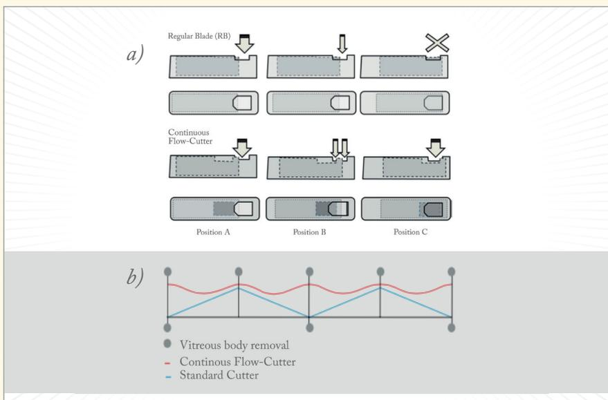
Figure 4. Standard cutter versus the OS4's Continuous Flow-Cutter. a) The Continuous Flow-Cutter always has at least half of the port open, and the blade cuts in both directions, doubling the cut rate. b) The Continuous Flow-Cutter (red) gives rise to continuous flow without noticeable fluctuations (as with each cycle, the vitreous body is removed twice), compared with the Standard Cutter (blue), where flow is interrupted each cycle, with vitreous body being removed only once per cycle
