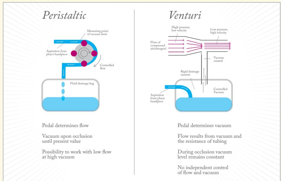
Figure 1. The conceptual differences between peristaltic and Venturi pumps.
